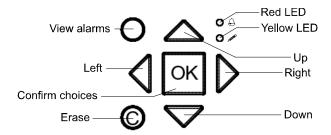
There are seven buttons: four arrow buttons which will be called UP, DOWN, RIGHT and LEFT. The menus in the Corrigo are organized in a horizontal tree structure. The UP/DOWN buttons are used to move between menus at the present menu level. The RIGHT/LEFT buttons are used to move between menu levels. When changing parameters the UP/DOWN buttons are used to increase/decrease the value of the parameter and the RIGHT/LEFT buttons to move between digits within the parameter.
