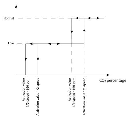
If demand controlled ventilation is activated in combination with mixing dampers, and the CO<sub>2</sub>-value rises above the setpoint value, the dampers will let in more outdoor air. The function is controlled by a PI-controller. See section 5.1.3 Heat exchanger types.
